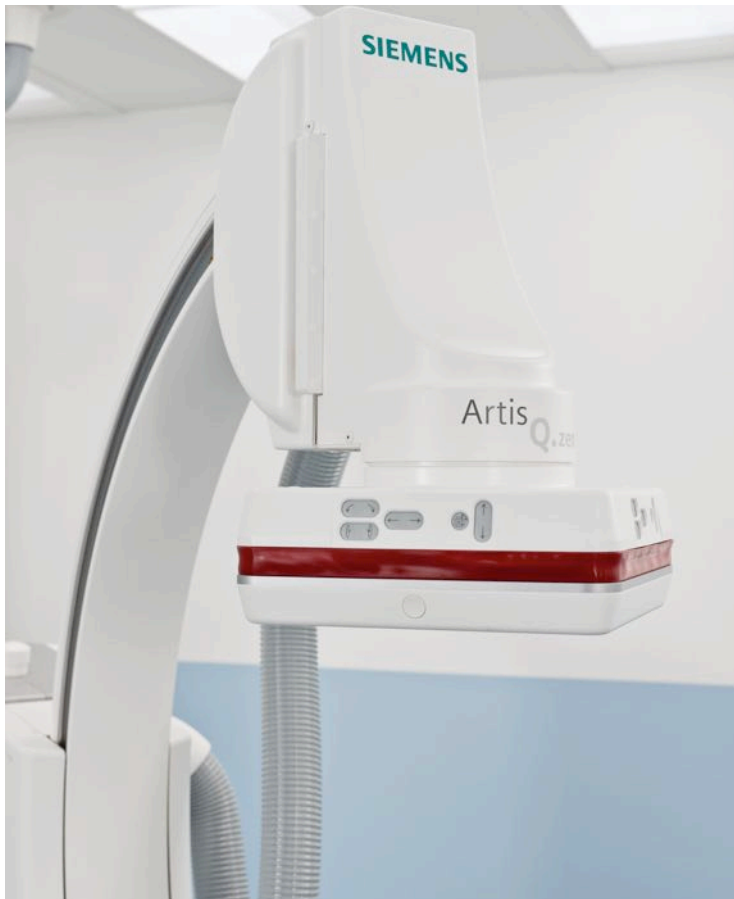
Figure 1. Artis Q.zen Crystalline Silicon FPD designed to allow ultra-low dose imaging.
